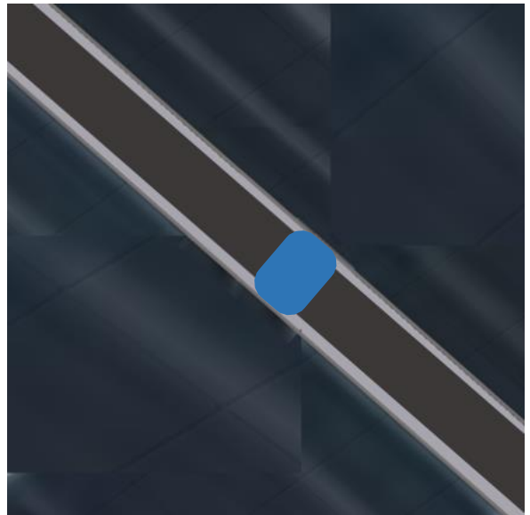
Use a copious amount of Sealant in and around the butt joint. Remove excess Sealant from panel glass.
