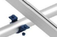
Attach the rail to the pipe using the aluminum pipe clamp kit. To prevent galvanic reaction, the PVC insulator must be installed be-tween the steel pipe and the aluminum rail.
