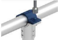
Position the Pipe Cap on top of the vertical pipe and lay the horizontal pipe into the Pipe Cap assembly.
