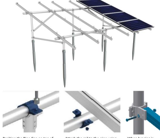
Position the Pipe Cap on top of the vertical pipe and lay the horizontal pipe into the Pipe Cap assembly. Attach the rail to the pipe using the aluminum pipe clamp kit. To prevent galvanic reaction, the PVC insulator must be installed be-tween the steel pipe and the aluminum rail. When bracing is required to a post, the pipe clamp kit is used.
