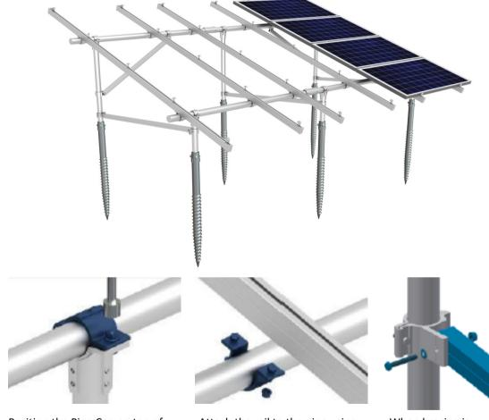
Position the Pipe Cap on top of the vertical pipe and lay the horizontal pipe into the Pipe Cap assembly.
