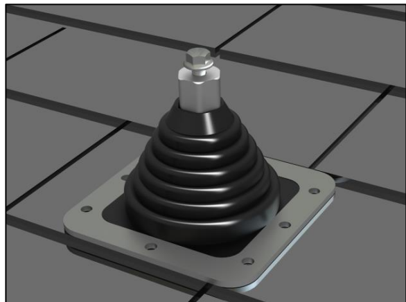
Step 4: Install a Rubber Roof Boot over the Standoff and secure using Sealant and small Teks screws.
